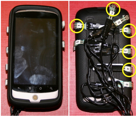
Figure 4: Nexus One phone in a protective case with force sensing resistors attached around its edges. The sensors used during the map task are circled.
